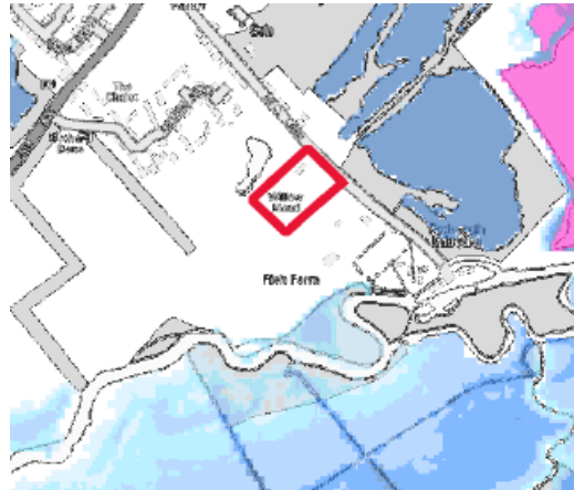
Figure 2: Flood depth mapping for 1 in 1000 year return period (0.1%AEP) from Willowmead FRA
