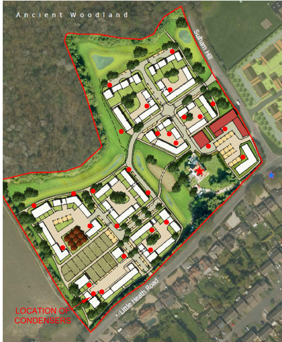
INDICATIVE LOCATION OF HEAT PUMP CONDENSERS
