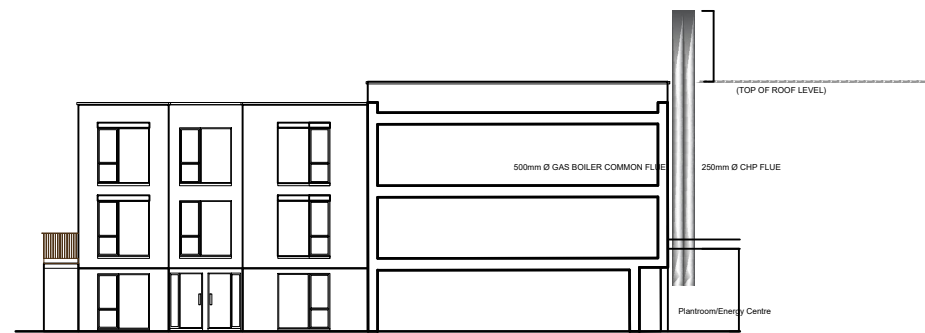
TYPICAL ENERGY CENTRE SECTION
