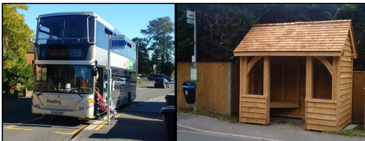
Figure 7.2 – Level boarding and new bus shelters
