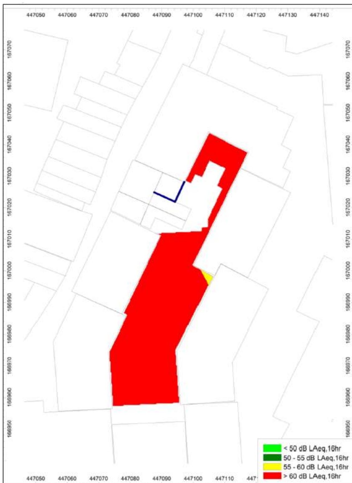
Figure 2. Acoustic model indicating that the predicted entertainment noise levels in the communal gardens surrounded by Blocks B, E and F will exceed the target set out by WHO (55 dB LAeq,T).
